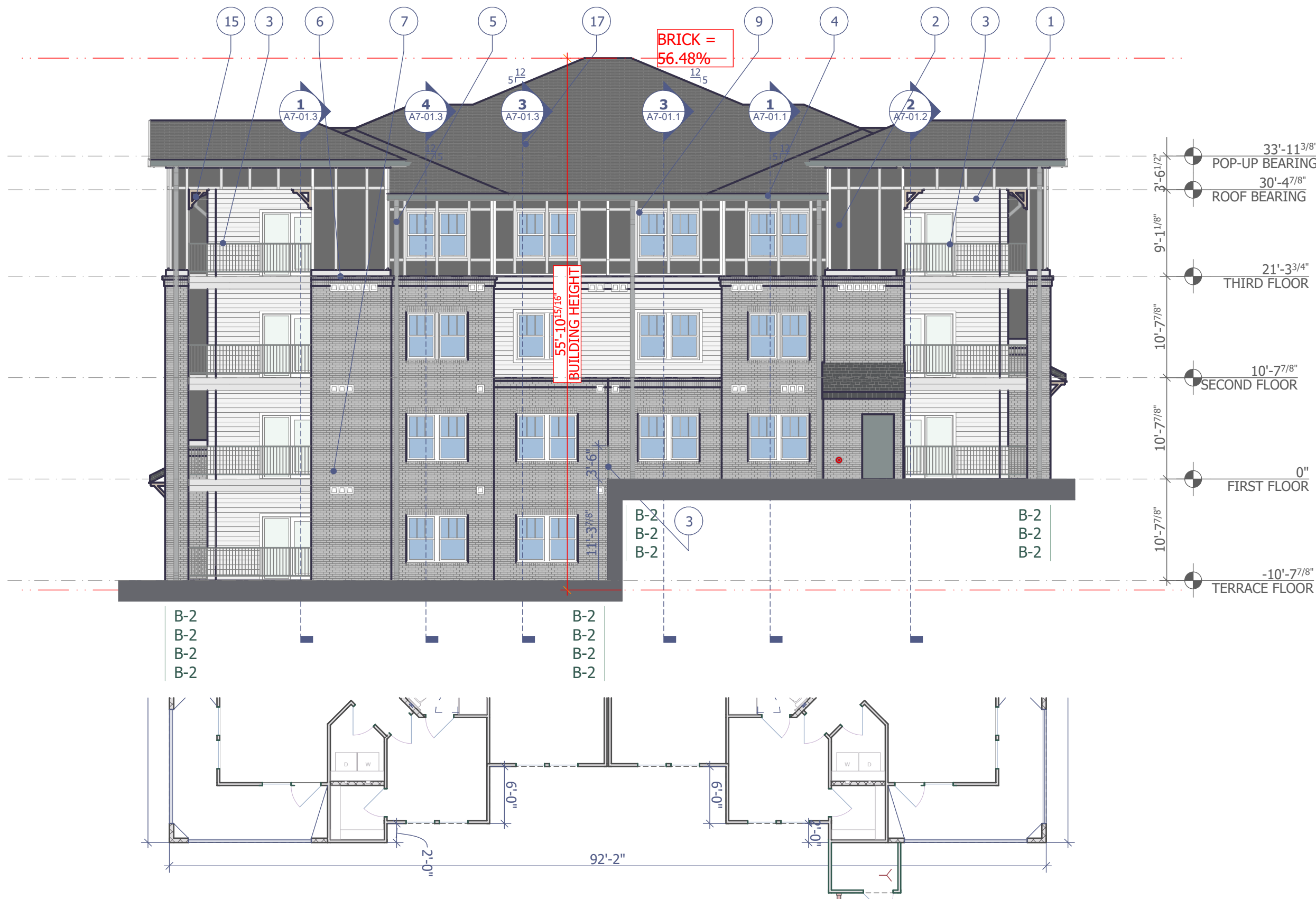
2 BLDG TYPE IV - 6000 RIGHT SIDE ELEVATION
